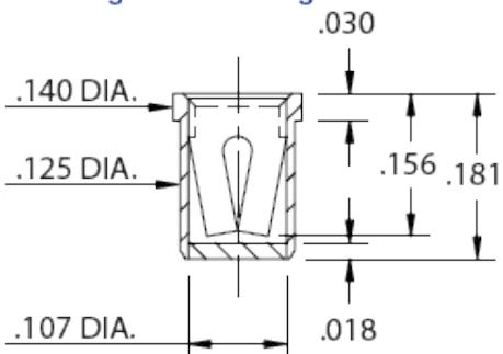
**0376-0-XX-XX-07-XX-10-0**Solder mount in  $\varnothing 0.133 \pm 0.003$  PTH.#07 Contact for  $\varnothing 0.065$ -.082 pins.
