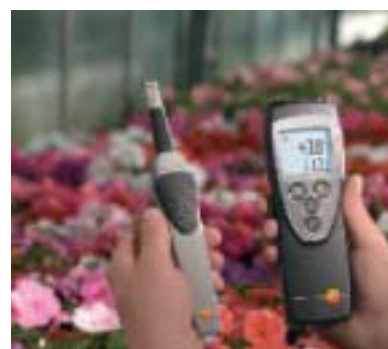
Moisture probe head attached to radio handle, e.g. for monitoring climate regulation
