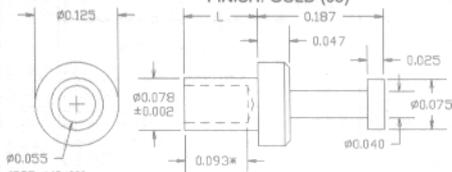
RECOMMENDED MOUNTING HOLE .082 DIA. (#45 DRILL)
