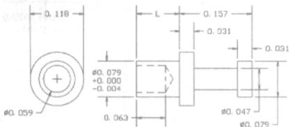
RECOMMENDED MOUNTING HOLE .081 DIA. (#46 DRILL)
