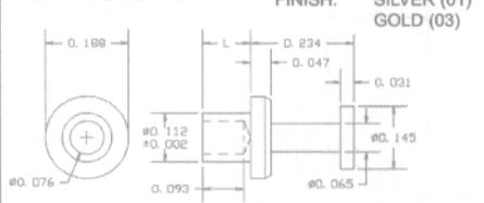
RECOMMENDED MOUNTING HOLE .116 DIA. (#32 DRILL)
