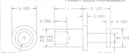
RECOMMENDED MOUNTING HOLE .094 DIA. (#32 DRILL)
