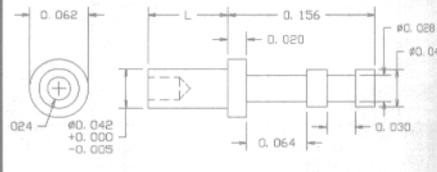
RECOMMENDED MOUNTING HOLE .043 DIA. (#57 DRILL)
