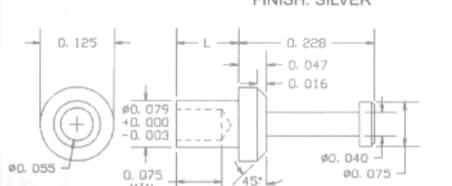
RECOMMENDED MOUNTING HOLE .082 DIA. (#45 DRILL)
