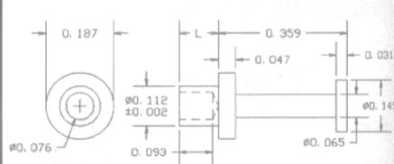
RECOMMENDED MOUNTING HOLE .116 DIA. (#32 DRILL)
