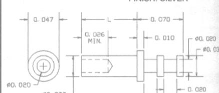
RECOMMENDED MOUNTING HOLE .043 DIA. (#57 DRILL)
