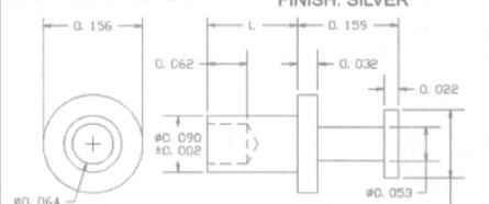
RECOMMENDED MOUNTING HOLE .094 DIA. (#32 DRILL)
