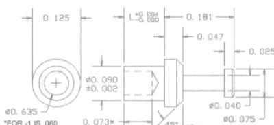
RECOMMENDED MOUNTING HOLE .094 DIA. (#32 DRILL)
