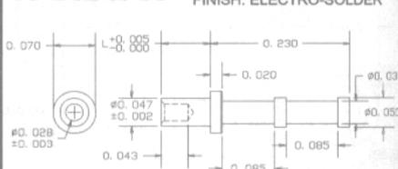
RECOMMENDED MOUNTING HOLE .052 DIA. (#55 DRILL)
