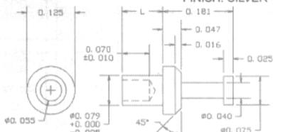
RECOMMENDED MOUNTING HOLE .082 DIA. (#45 DRILL)
