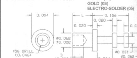
RECOMMENDED MOUNTING HOLE .067 DIA. (#51 DRILL)
