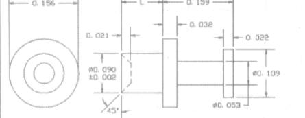
RECOMMENDED MOUNTING HOLE .094 DIA. (#42 DRILL)
