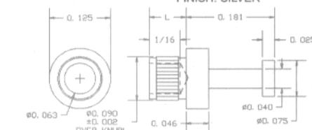
RECOMMENDED MOUNTING HOLE .094 DIA. 3/32 DRILL)
