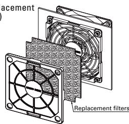
● Replacement filters can be replaced by taking off the front part of the filter kit. There is no need to remove the screws.
