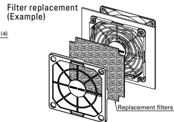
● Replacement filters can be replaced by taking off the front part of the filter kit. There is no need to remove the screws.
