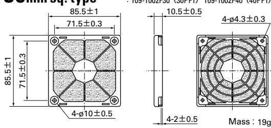
**Material** Guard, cover : Resin (PPE+PS) UL File No.E82268 94V-1
