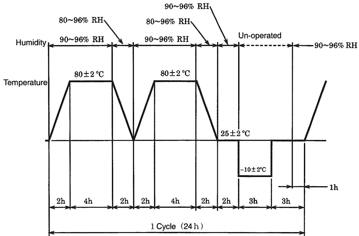
Fig. 9 Humidity-Temperature Cycling
