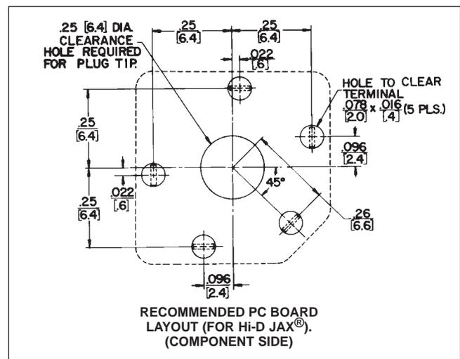
DIMENSIONS ARE FOR REFERENCE ONLY  $\frac{\text{Inch}}{\text{(mm)}}$
