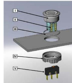
During assembly, the protruding bars of the holder should not be pressed together.
