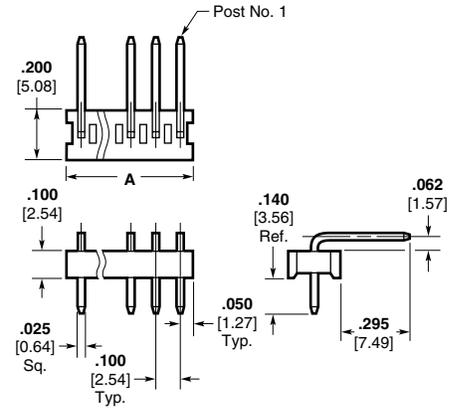
X = .120 [3.05] min., .240 [6.1] max. when mated with MTA-100 Connector.
