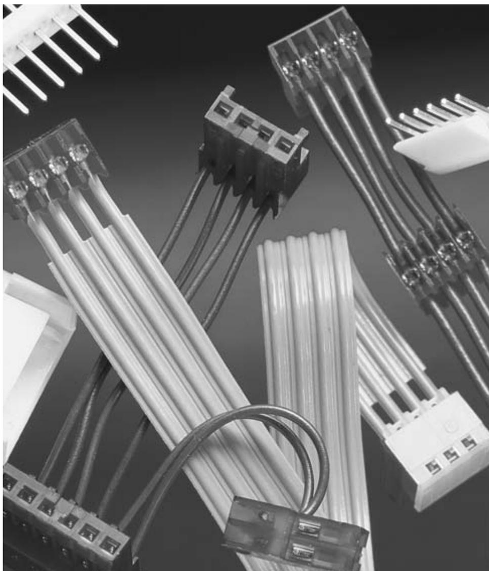
MTA-100 connectors accept discrete and ribbon cable wire sizes ranging from 22–28 AWG [0.4–0.08 mm<sup>2</sup>] with maximum insulation outside diameter of .060 [1.52] for terminating single wire and .050 [1.27] for mass termination of wires. Tin plated solid, fused stranded, or stranded (7 strands) wire with PVC insulation can be used on 22–28 AWG [0.4–0.9 mm<sup>2</sup>] MTA-100 connectors and 19 stranded wire on 22–24 AWG [0.4–0.2 mm<sup>2</sup>] MTA-100 connectors. Only
