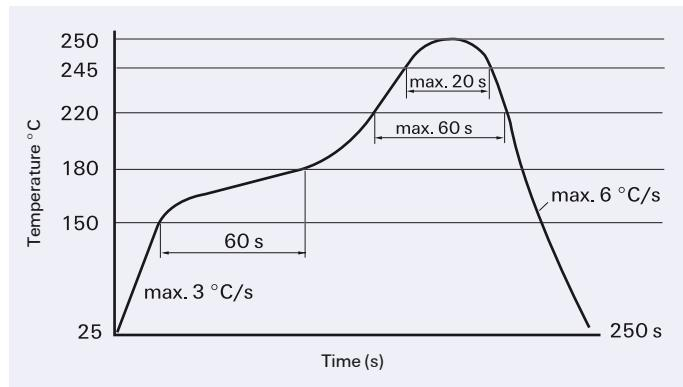
Infrared Soldering: Temperature/Time Profile
