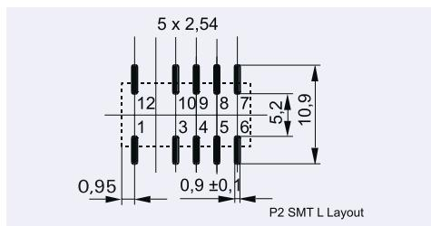
Note: Solder pad for pin 6 and 7 only for latching with 2 coils
