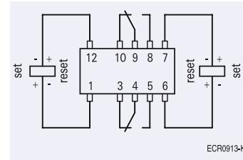
Contacts in reset position. Both coils can be used either as set or reset coils.
