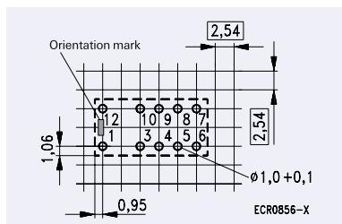
Note: Hole for pin 6 and 7 only for latching with 2 coils. Basic grid 2.54 mm
