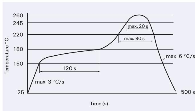
Infrared Soldering: Temperature/Time Profile
