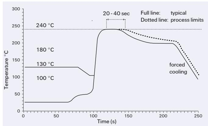
Vapor Phase Soldering: Temperature/Time Profile
