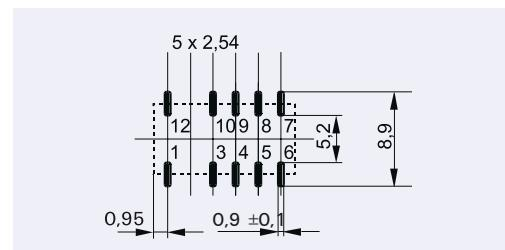
Note: Solder pad for pin 6 and 7 only for latching with 2 coils
