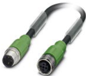
Sensor/Actuator cable, 3-position, PUR halogen-free, black-gray RAL 7021, shielded, Plug straight M12, A-coded, on Socket straight M12, A-coded, Cable length: 0.3 m
