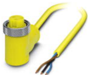
Sensor/Actuator cable, 3-position, PVC, Yellow RAL 1021, free cable end, on Socket angled 7/8"-16UNF, A-coded, Cable length: 4 m
