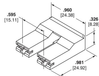
Two Circuit Water Valve Housing
