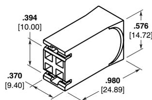
Two Circuit Wax Motor Housing
