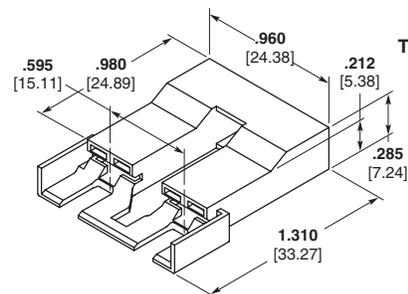
Two Circuit Water Valve Housing
