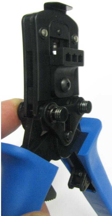
Picture 1: Pressing out the locking pins from the front
