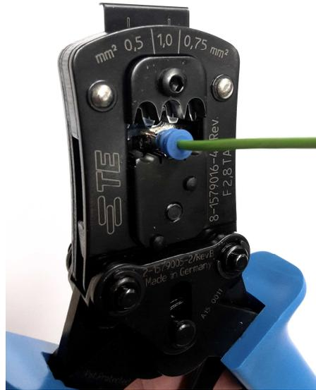
Picture 8: Insert the wire with the sealing ring
