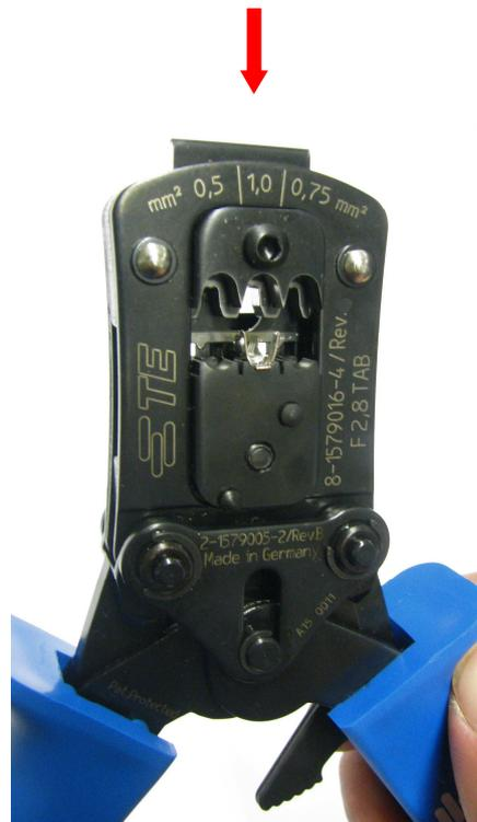
Picture 6: Push the sliding positioner downwards
