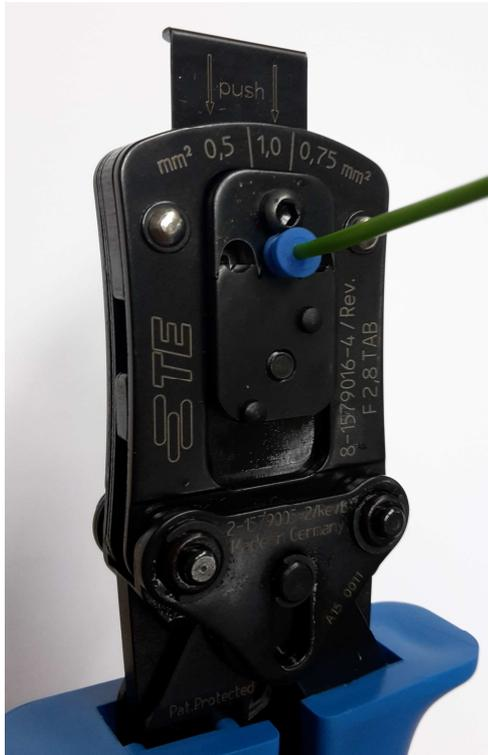
Picture 9: Closed crimp tool (crimping head)
