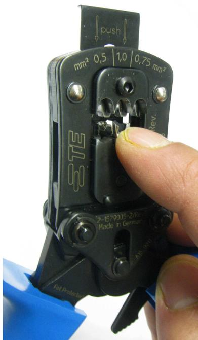
Picture 5: Inserting the contact
