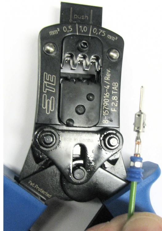
Picture 10: Checking the crimping contact
