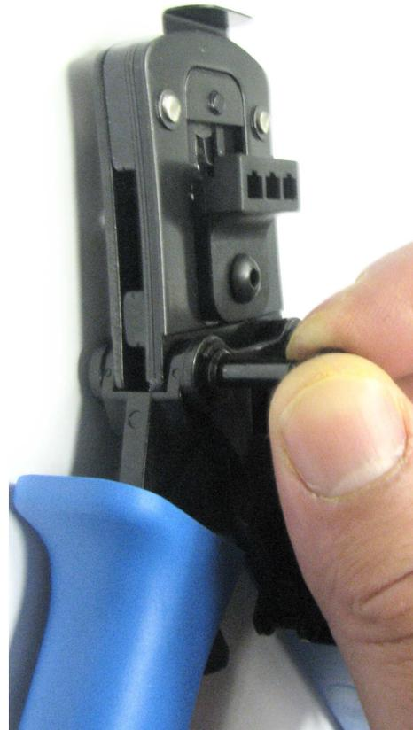
Picture 2: Removing the locking pins
