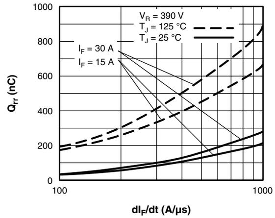
Fig. 8 - Typical Stored Charge vs.  $di/dt$
