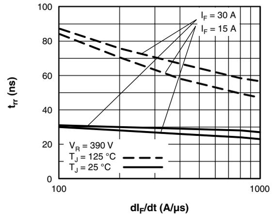
Fig. 7 - Typical Reverse Recovery vs.  $di/dt$
