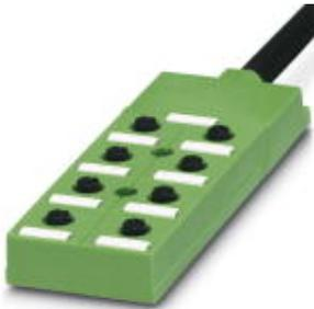
Sensor/actuator box, Connection method: M12 socket Plastic, Number of slots: 6, Number of positions: 5, Slot assignment: Double, Status indication: No, Universal; Master cable connection: Fixed connection 180°, PUR/PVC, Cable length: 10 m, Shielding: No
