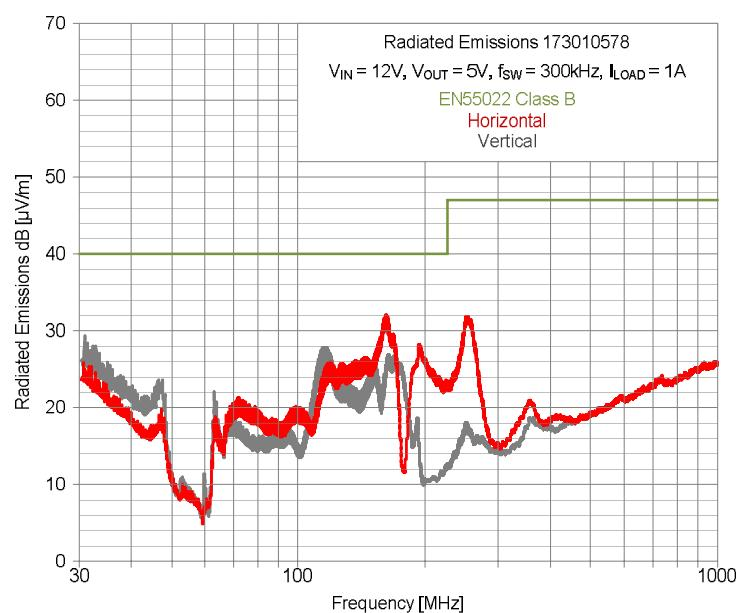
Measured without external filters at 3m antenna distance
