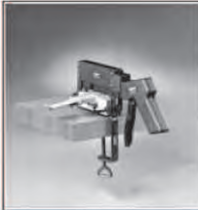
Pistol Handgrip Tooling. This is a handtool for terminating Micro-MaTch Male-on-Wire and Paddle Board connectors. Meant for small quantities or repair services. Pistol handgrip and adapter must be ordered separately.
