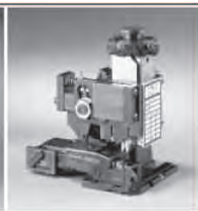
Applicators for AMP-O-ELECTRIC G-terminator. Part Number 677894-1 for AWG 28-24 (Part Number 338096-1) and Part Number 677895-1 for AWG 24-20 (Part Number 338097-1).
