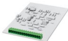
Header, Nominal current: 12 A, Rated voltage (III/2): 320 V, Number of positions: 15, Pitch: 5.08 mm, Color: green, Contact surface: Tin, Mounting: Soldering
