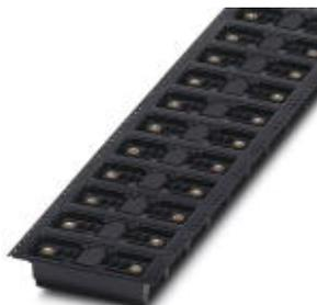
Header, Nominal current: 8 A, Rated voltage (III/2): 160 V, Number of positions: 7, Pitch: 3.5 mm, Color: black, Contact surface: Tin, Mounting: Taped SMD/THT/THR components, User information and design recommendations for through hole reflow technology can be found under "Downloads"
