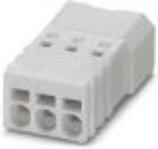
Plug component, nominal current: 6 A, rated voltage (III/2): 160 V, number of positions: 5, pitch: 2.5 mm, connection method: Push-in spring connection, Color: white, Contact surface: Tin
