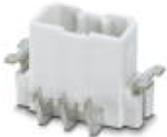
Header, nominal current: 6 A, rated voltage (III/2): 160 V, number of positions: 5, pitch: 2.5 mm, Contact surface: Tin, mounting: SMD soldering
