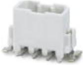
Header, nominal current: 6 A, rated voltage (III/2): 160 V, number of positions: 5, pitch: 2.5 mm, Color: white, Contact surface: Tin, mounting: SMD soldering, Article with anti-rotation pin
