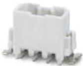
Header, nominal current: 6 A, rated voltage (III/2): 160 V, pitch: 2.5 mm, Color: white, Contact surface: Tin, mounting: SMD soldering
