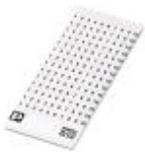
Marker card, Card, white, labeled, Horizontal: Consecutive numbers 1 - 10, 11 - 20, etc. up to 91 - 99, Mounting type: Adhesive, for terminal block width: 3.5 mm, Lettering field: 3.5 x 2.8 mm
