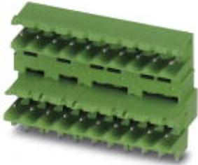
Header, Nominal current: 10 A, Rated voltage (III/2): 320 V, Number of positions: 9, Pitch: 5.08 mm, Color: green, Contact surface: Tin, Mounting: Wave soldering, The article can be aligned to create different nos. of positions! In combination with MVSTB or FKCV plug components, both an MVSTBW (or FKCVW) and an MVSTBR plug (or FKCVR) must be used. Combination with TMSTBP plug components is not possible!
