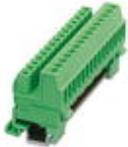
Plug component, Nominal current: 12 A, Rated voltage (III/2): 320 V, Number of positions: 9, Pitch: 5.08 mm, Connection method: Screw connection with tension sleeve, Color: green, Contact surface: Tin, Mounting: DIN rail
