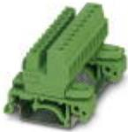
Plug component, Nominal current: 12 A, Rated voltage (III/2): 320 V, Number of positions: 9, Pitch: 5.08 mm, Connection method: Screw connection with tension sleeve, Color: green, Contact surface: Tin, Mounting: DIN rail
