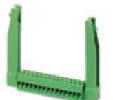
Plug component, Nominal current: 12 A, Rated voltage (III/2): 320 V, Number of positions: 9, Pitch: 5.08 mm, Connection method: Screw connection with tension sleeve, Color: green, Contact surface: Tin, Mounting: Direct mounting
