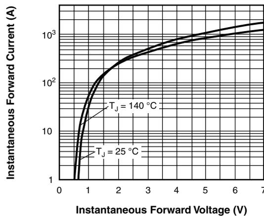
Fig. 5 - Maximum Forward Voltage vs. Forward Current
