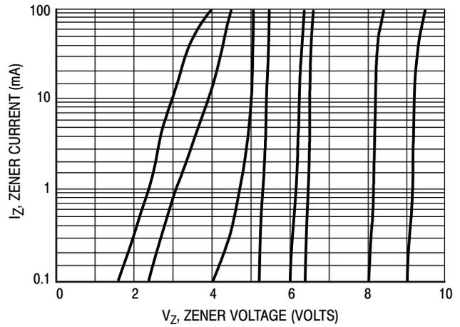
Figure 2.  $V_Z$  - 3.3 thru 10 Volts
