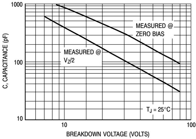
Figure 7. Capacitance Curve
