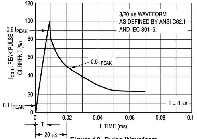
Figure 10. Pulse Waveform
