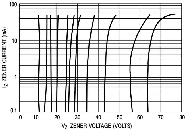
Figure 3.  $V_Z = 12$  thru 68 Volts
