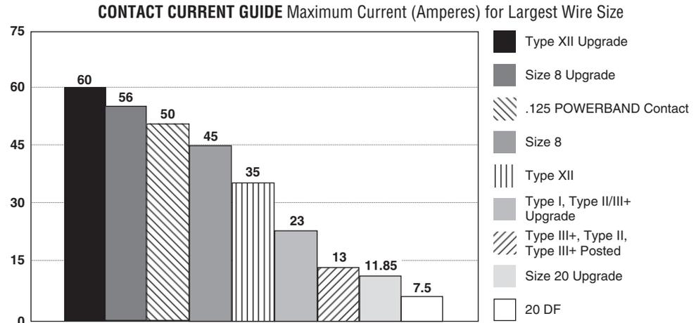
■ **Wire Size**—Larger wire will carry more current since it has less internal resistance to current flow and generates less heat. The wire also conducts heat away from the connector.
