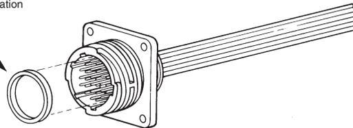
**Receptacles with pre-installed, bonded peripheral seals** are recommended for use in sealing/splash-proof applications, or where connectors will be subjected to vibration.
