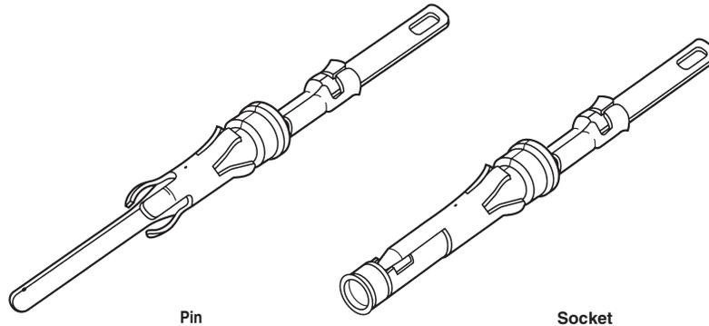
**Contact Size 16—Pin Diameter .062 [1.57] (Test Current, 13 Ampere)‡**
