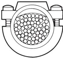
The clamping area can be adjusted by reversing the clamping insert as shown below.
