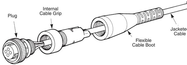
**Flexible Cable Boot and Internal Cable Grip (for Shell Size 17)**
