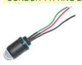
2 colour LED (3 wires) Steady Red and Steady Green. Fits to conduit entry of most switches and provides option for LED indication based upon switch contacts. The dome shaped LED is visible from narrow angles. Available voltages 24Vdc, 110Vac or 230Vac and either M20 or 1/2" NPT conduit thread. PVC conductors, fully encapsulated IP67. Maximum temperature: 60C. Housing material is polyester.
