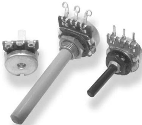
A popular range of 20mm control potentiometers, the type 23 series can be tailored to suit more specific requirements. The potentiometers are available with printed carbon resistance element, choice of bush lengths in metal or plastic and insulated shafts up to 50mm in length. In addition, approved mains and low current switches are available as standard options.
