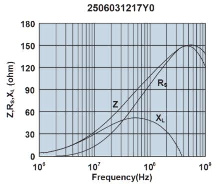
Impedance, reactance, and resistance vs. frequency.
