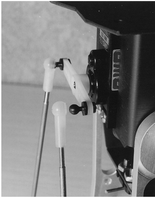
Figure 1-17 Install tilt rods.
