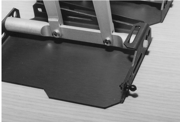
Figure 1-15 Install ball joints on feet.
