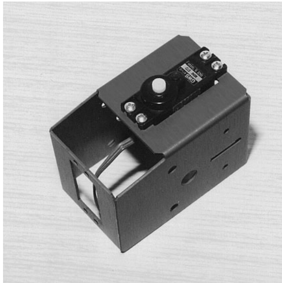
Figure 1-1 Install Tilt Servo in Body
