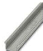
DIN rail, material: Steel, unperforated, 2.3 mm thick, height 15 mm, width 35 mm, length: 2 m
