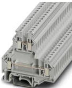
Feed-through terminal block, Cross section: 0.2 mm<sup>2</sup> - 4 mm<sup>2</sup>, AWG: 24 - 12, Connection type: Screw connection, Width: 6.2 mm, Color: gray, Mounting type: NS 35/7,5, NS 35/15, NS 32
