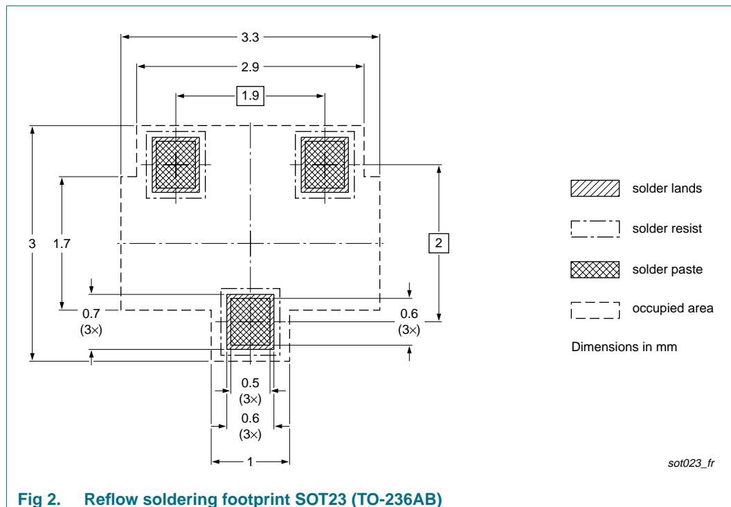
**Fig 2. Reflow soldering footprint SOT23 (TO-236AB)**
