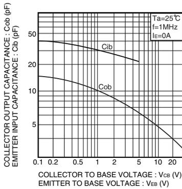
Fig.7 Input-and-output capacity vs. voltage characteristic
