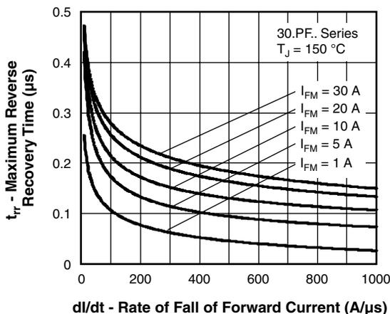
Fig. 9 - Recovery Time Characteristics,  $T_J = 150\text{ }^\circ\text{C}$
