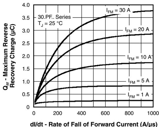
Fig. 10 - Recovery Charge Characteristics,  $T_J = 25\text{ }^\circ\text{C}$
