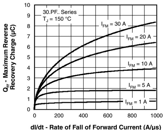
Fig. 11 - Recovery Charge Characteristics,  $T_J = 150\text{ }^\circ\text{C}$
