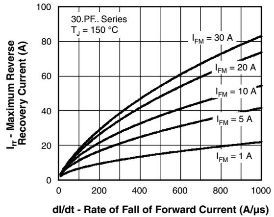
Fig. 13 - Recovery Current Characteristics,  $T_J = 150\text{ }^\circ\text{C}$
