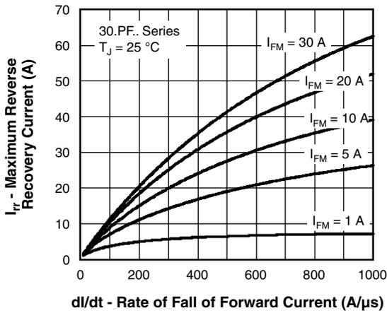
Fig. 12 - Recovery Current Characteristics,  $T_J = 25\text{ }^\circ\text{C}$
