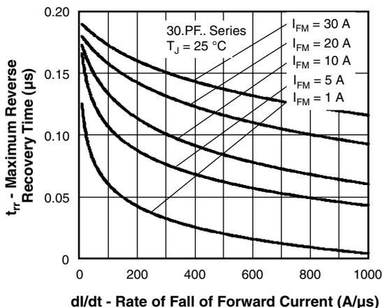
Fig. 8 - Recovery Time Characteristics,  $T_J = 25\text{ }^\circ\text{C}$
