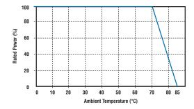
When the ambient temperature exceeds 70°C, reduce the rated power and current in accordance with the derating curve shown
