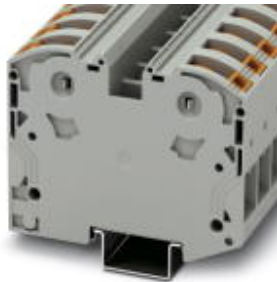
High-current terminal block, Connection method: Power-Turn connection, Cross section: 2.5 mm 2 - 35 mm 2 , AWG: 12 - 2, Width: 16 mm, Color: gray, Mounting type: NS 35/15
