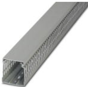
Cable duct, light gray, halogen-free, consisting of upper part and mounting base, width: 60 mm, height: 80 mm, length: 2000 mm
