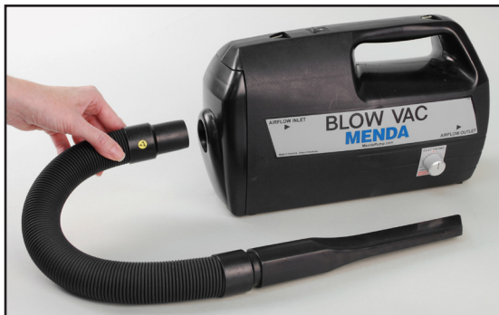
Figure 3: Connecting the hose to the airflow inlet.
