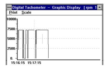
If this option is selected or CTRL+G is pressed, a window, which emulates strip chart recorder, shall appear on the screen. The graphic window has two menu, PRINT and SCALE. Select the PRINT menu, the graphics will be printed through any printer connected to the PC. The SCALE menu allows user to set the minimum and maximum value for the Y (vertical) axis.
