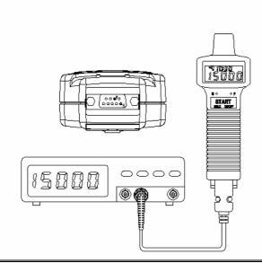
**NOTE:** It is strongly recommended that the emiting/receiving unit be covered to avoid undesired light signal coming in.
