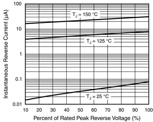
Figure 4. Typical Reverse Leakage Characteristics Per Diode
