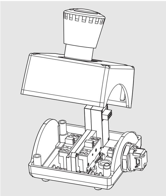
The enclosures with integrated AS-Interface are equipped with contact blocks and LED lampholders with spring-loaded terminals from the 3SB3 series along with the slave(s) required to connect the contact blocks and lampholders to AS-Interface.
