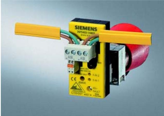
The AS-Interface F adapter is used to connect an EMERGENCY-STOP control device according to ISO 13850 or EN 418 from the 3SB3 series to the AS-Interface bus system.
