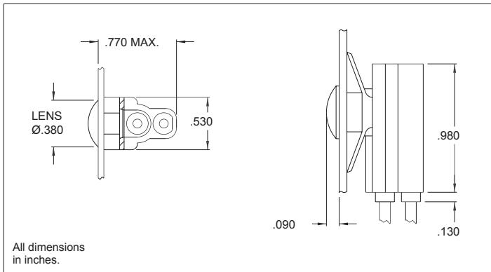
Mounting: Will snap-fit into Ø.032/.317 in panels .202/.125 thick.
