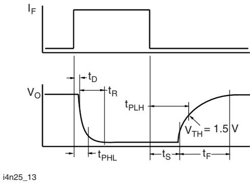
Fig. 13 - Switching Timing
