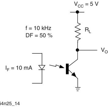
Fig. 14 - Switching Schematic
