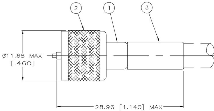
1. USE CRIMPING TOOL: PRO-CRIMPER WITH DIE SET 58494-1 OR DIE HOLDER 764593-1 WITH DIE SET 58494-1 IN CONJUNCTION WITH PNEUMATIC TOOLS, 314281-1, 314700-1, 314590-1, 314590-2, OR 856402-1
