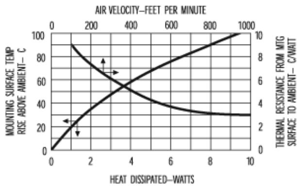
Thermal resistance value is based on a 75°C rise in natural convection
