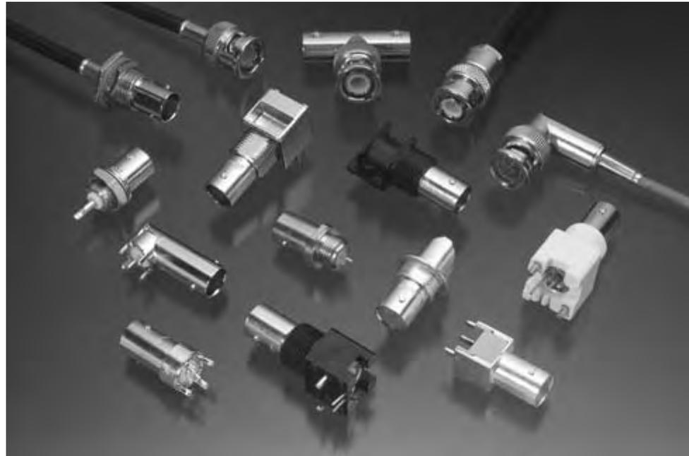
The Tyco Electronics BNC RF connector family with bayonet locking coupling provides highly reliable, quick connect/disconnect coaxial connections. Exclusive single and O crimp terminations allow positive insulation grip and require no soldering, providing terminations at a very low overall applied cost.
