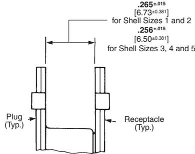
The .265 [6.73] dimension is required to assure full mating of connector halves. This dimension must be taken into consideration when determining the method of mounting, panel thickness, etc.
