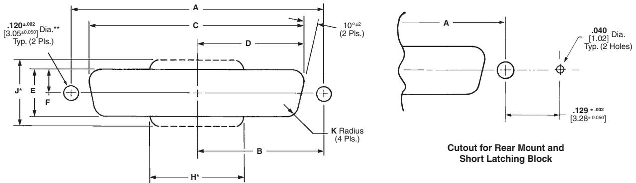
**Note:** Cutouts are for either plug or receptacle, front or rear panel mount.
