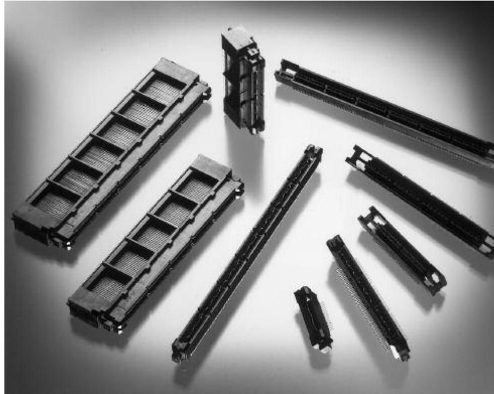
The MICTOR connector family is based on the microstrip concept of two rows of signal contacts divided by a center power ground plane. MICTOR connectors are mother-board and daughtercard compatible and include designs for cable-to-board applications.
