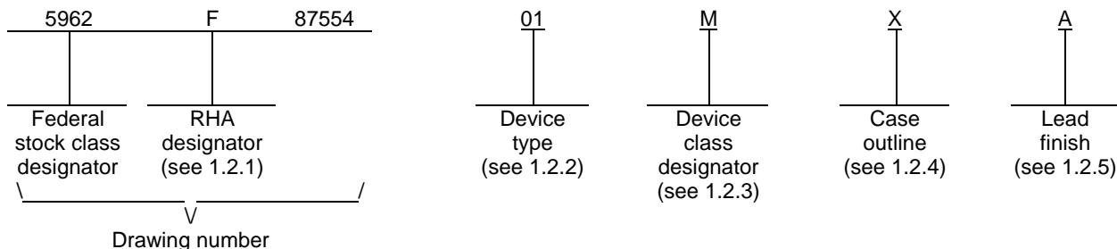
1.2.1 RHA designator. Device classes B, S, Q, and V RHA marked devices meet the MIL-PRF-38535 specified RHA levels and are marked with the appropriate RHA designator. Device class M RHA marked devices meet the MIL-PRF-38535, appendix A specified RHA levels and are marked with the appropriate RHA designator. A dash (-) indicates a non-RHA device.
