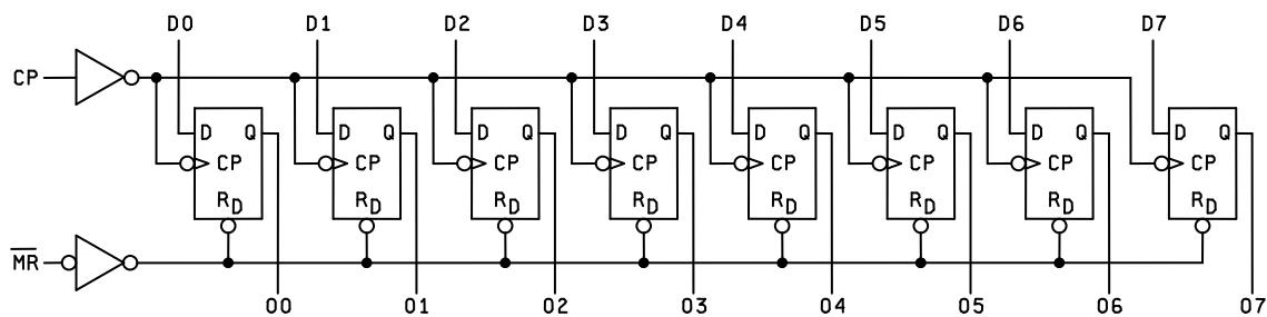
FIGURE 3. Logic diagram.
