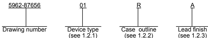
1.2.1 Device type(s). The device type(s) identify the circuit function as follows:
